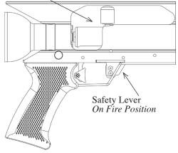
⚠ WARNING: Do not move the safety to the On Fire position unless the air gun is pointed in a safe direction. Safe means that if the gun discharged it would not cause injury or property damage. Mechanical safeties are not infallible and do not replace the need for responsible gun handling practices.
